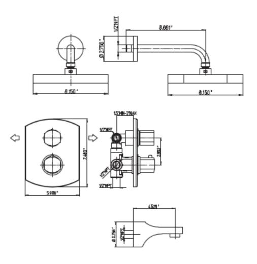
Novello thermostatic valve with 2-way diverter volume control ½" inlet connections
