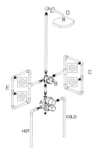
Lady thermostatic valve with 3/4" ceramic disk volume control 8" rain shower head with 12" arm 3-way diverter 3 concealed body jets
