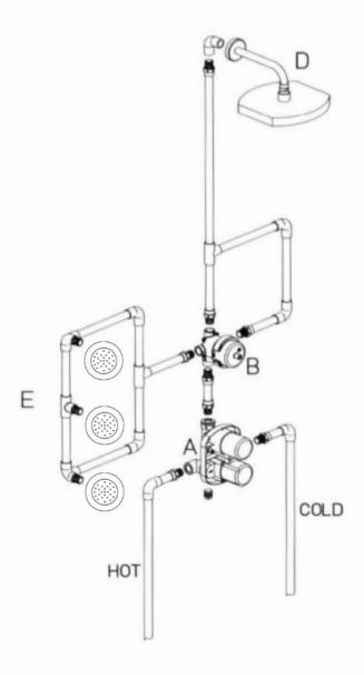
Novello thermostatic valve with 34" ceramic disk volume control 8" rain shower head with 12" arm 3-way diverter 3 concealed body jets
